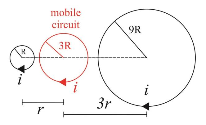
Experimental observation: The mobile circuit remains at rest.
