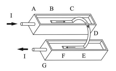
According to Ampère, the observed force on the bridge pointing towards the right is due to the repulsion between portions AB and BC, together with the repulsion between portions EF and FG.
