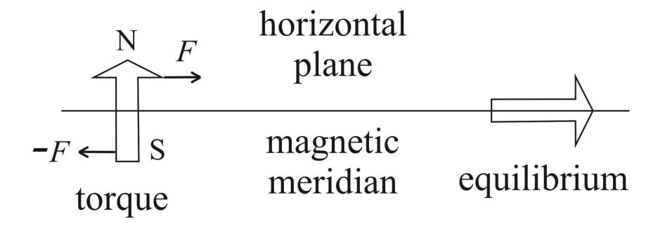
Ampère's 1820 experiment showing an electrodynamic analogue of the directive torque exerted magnetically by the Earth on a compass needle. The current carrying loop can turn around its vertical axis of symmetry. The Earth exerts an electrodynamic torque on the current loop.
