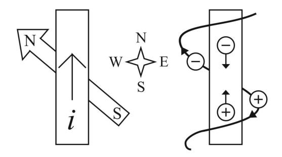
"Negative electricity propels the North pole, but does not act on the South pole. Positive electricity propels the South pole, but does not act on the North pole." Biot and Savart's interpretation (1820) of Oersted's experiment:
