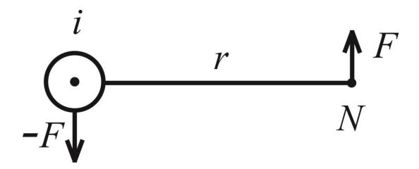
These transverse forces would generate an internal or primitive couple (torque) on the system.
