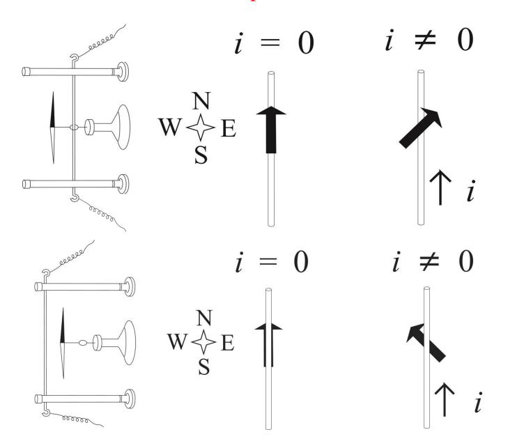
Oersted's interpretation based on the helical flow of charges <u>outside</u> the current carrying wires.
