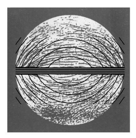
Experimental lines of electric field compared with theoretical calculations. Equipotentials measured with an electrometer in a hollow rectangular chamber with graphite paper (I =  $5x10^{-2}$  A) or photographic film (I =  $4x10^{-6}$  A) on the walls. Jefimenko et al., Proc. West Virginia Acad. Sci. <u>34</u>, 163 (1962).
