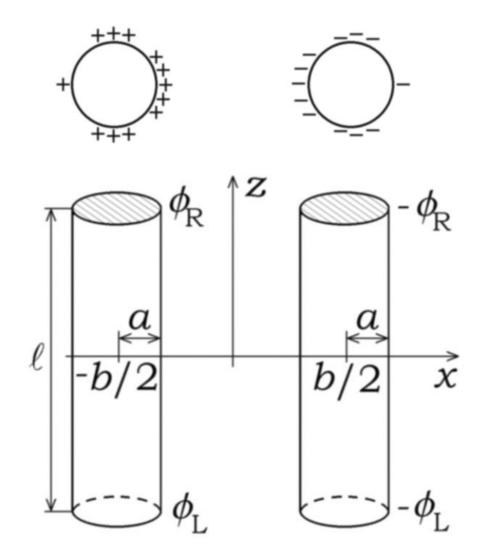
Experiments by Bergmann, Schäfer and Jefimenko for a transmission line showing the external electric field, compared with theoretical solution:
