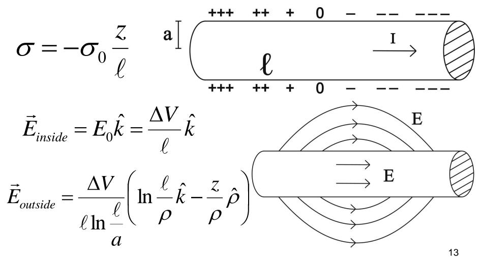
**Experiment** by Bergmann and Schäfer (Elektrizität und Magnetismus, 1950). Constant current flowing along a high resistance paper strip surrounded by oil with semolina.  $\Delta V = 30$  kV.
