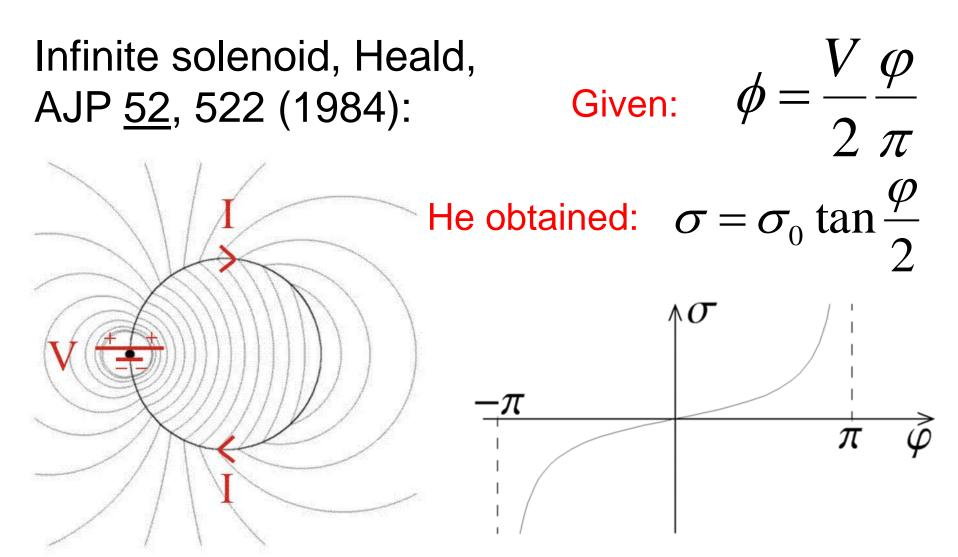
E outside  $\neq$  0. Moreover, the density of surface charge does not vary linearly with the azimuthal angle.
